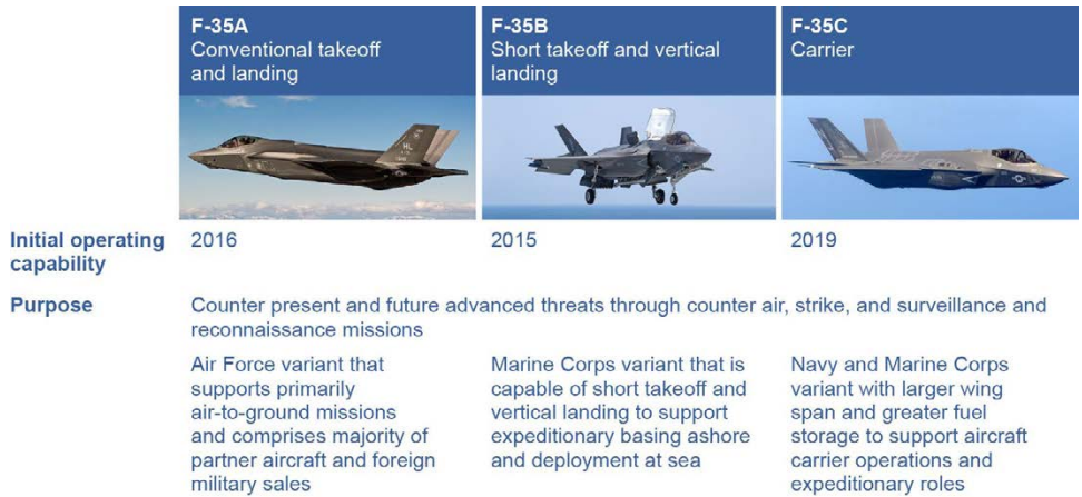
Figure 2: Variants of the F-35 Aircraft
