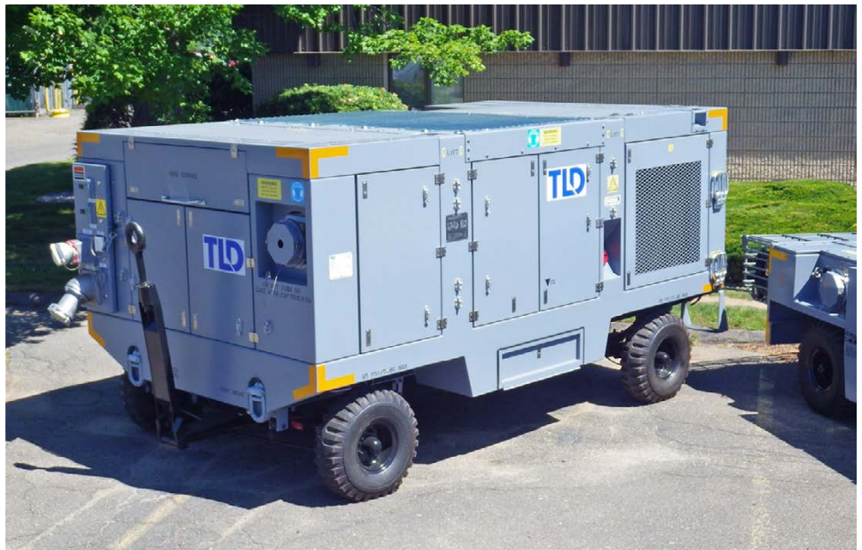
Figure 10: Conditioned Air Cart for the F-35's Power and Thermal Management System
